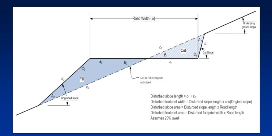
Exploration Road - 14 feet running width At 5% Slope – disturbance width of 15 feet At 15% Slope – disturbance width of 17 feet At 25% Slope – disturbance width of 19 feet
